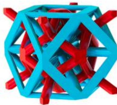
Abb.1: Interpenetrating Lattice aus FCC+RD [1]
