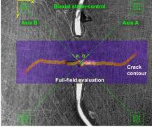
Due to the random orientation of the cracks, crack tip detection currently still requires manual post-processing. The aim of this thesis is therefore to develop an algorithm in Python that can find the crack tip using existing strain data from a test sample and reproduce the course of the crack in a robust manner.
