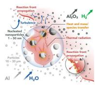
Micron sized metal powder can serve as a carbon free energy carrier in a circular energy economy, in a similar manner as hydrogen. Energy is stored by reducing aluminum ore to aluminum. The  $CO_2$ -free combustion of aluminum particles suspended in pure steam (H<sub>2</sub>O) is one possible thermochemical process to release the stored energy, obtaining around half of the energy in the form of heat and hydrogen gas, respectively.
